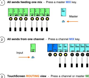
TouchScreen ROUTING view - Press a channel or master SEL key while the TouchScreen ROUTING page is active.
